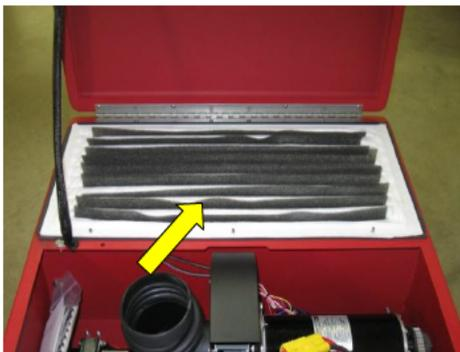
The 34 sweeper uses “baghouse” filter made of poly felt. The poly material lasts longer than disposable paper and the felt pattern offers superior filtration. It can be cleaned and used for years, not like the less expensive paper options. Our intent is that this will save the customer money.
