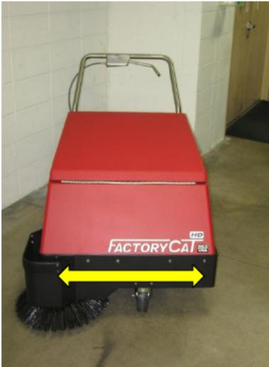
The heavy duty wide steel frame of the 34 sweeper offers stability without the need for tip-over bars used on some other machines.
