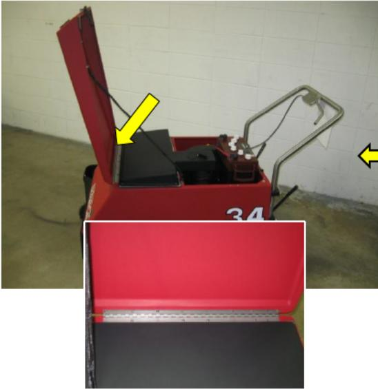
The 34 sweeper uses a large stainless hinge for the hood that bolt directly to the steel frame. This provides better durability than other machines that use smaller hinges bolted to plastic frames.
