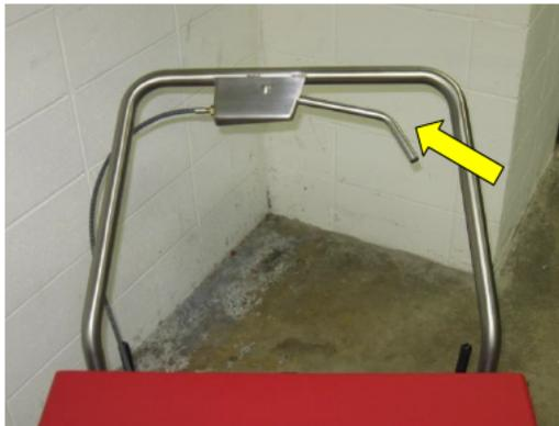
The 34 sweeper has a large lever to control the speed. The large lever makes it easy for all users to be able to grip it. It also serves as the brake control when pushed down.
