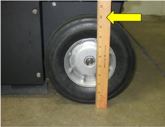
TR sweeper 's have a 10" diameter tire. The large diameter improves the ride over expansion joints and irregular concrete surfaces. Each tire is rated at 1,500 lbs, which is 3 times greater than the load of the machine with a full hopper.
