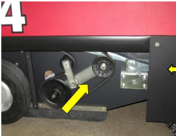
The 34 sweeper uses durable, heavy-duty steel trailing arms and in a "Trailing Arm" manner. The steel arms hold up to years of use and the trailing arm allows the broom to float over the floor. This eliminates the need to "reverse" the broom regularly and the use of a V broom pattern, which fills the hopper from the center out.
