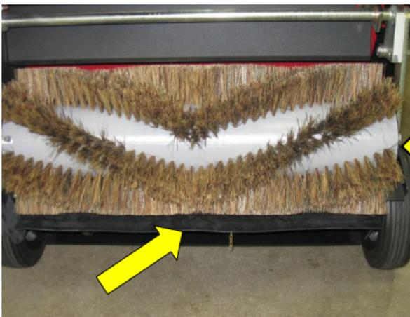
The 34 employs an attenuator flap, recycling flap and rear air control curtain. The attenuator flap keeps debris from cycling over the broom, while the recycling flap helps direct debris back into the broom. The air control curtain manages airflow from the back of the machine, and improves dust control.
