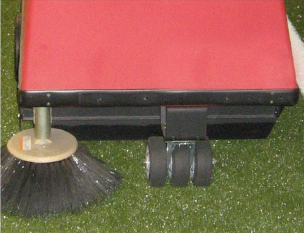
← Artificial Turf Grooming Package is a unique set of components that allow the sweeper to nicely groom and sweep many artificial turf types. The option includes: Extra wide front caster wheels (triple wheels) Special Seal Option Full pack nylon broom
