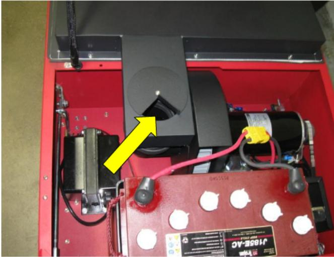
A feature to 34 sweeper is the Wet Sweep ByPass door. The operator can simply rotate this cover open to reduce the airflow into the filter when water on the ground is encountered.
