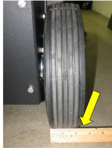
Our 34 sweeper 2.5" rear HD tires are wider than tires on many other machines. The additional width increase traction and stability. The 34 also offers a softer footprint (lower psi) than machines with smaller tires and is friendly to sensitive ceramic tile edges, carpeting or artificial turf in sports arenas.
