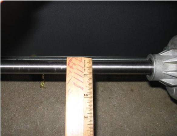
The 34 sweeper 1" axle is larger than axles on many other machines. The larger axle is designed to support the unit in harsh applications and last the life of the machine.
