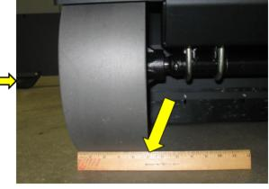
The TR sweeper 2" axle is larger than axles on many other machines. The larger axle is designed to support the unit in harsh applications and last the life of the machine.
