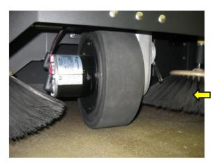
HD Front Drive Available as an upgrade over the standard 1.0 hp (10" diameter) front wheel drive. The 2.0 hp motor is better able to climb steep ramps and the larger 12" diameter and 4" wide tire will operate better over rough floors.
