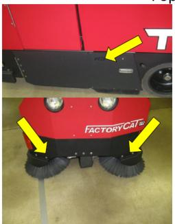
Side Doors are heavy gage, powder painted steel doors, which hinge open to access the main broom and belts. These HD doors mount with a stainless hinge, to the rider's steel frame, and protect from collisions into poles, pallets and such. Also side broom guards made with the same 7 gauge steel are avialable with the HD package.
