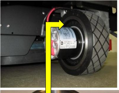
The components on the left side are from the Front Wheel "Chassisdrive" used on the TR sweeper. This drive is built in the Mid-West of the USA and with much stronger components. The stars point out the difference between our drive and the cheaper import (Asia and Europe) that is used on some competitors. The major difference being the size and therefore the strength.
