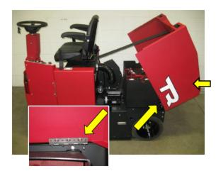
The TR sweeper uses larger (8" stainless) hinges, a steel hood and bolt directly into the heavy gage steel frame. This provides better durability than other machines that use smaller hinges bolted to plastic covers.
