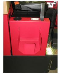
Operator's Side tray for weed spray bottle. Ideal for holding a 2 gallon pump sprayer. This small platform is easily installed or removed without tools.
