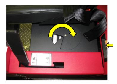
A handy feature on the TR sweeper is the Wet Sweep ByPass door. The operator can simply rotate this cover open to reduce the airflow into the filter when water on the ground is encountered.
