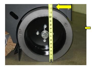
TR sweeper 's have 14" diameter rear tires. The large diameter improves the ride over expansion joints and irregular concrete surfaces. Each tire is rated at 2,200 lbs, which is 3 times greater than the load of the machine with a full hopper.
