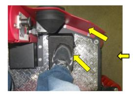
The TR sweeper has a simple and large pedal, which controls speed. This view also shows the protection offered to the Operator's foot on the TR sweeper . A complete apron across the front makes it harder for the operator to hang a foot off the side, reducing operator injuries. Separate forward/reverse switch improves control and reduces wear on motors, tires, and skid marks.
