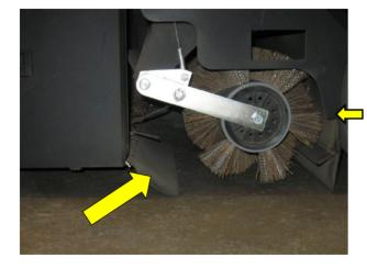
The TR employs an attenuator flap, recycling flap and rear air control curtain. The attenuator flap keeps debris from cycling over the broom, while the recycling flap helps direct debris back into the broom. The air control curtain manages airflow from the back of the machine, and improves dust control.
