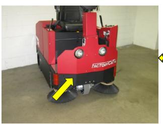
The TR sweeper has a heavy duty steel frame – not plastic like some other machines – for durability and protection. The heavy duty wide steel frame of the TR sweeper offers stability without the need for tip-over bars used on some other machines.
